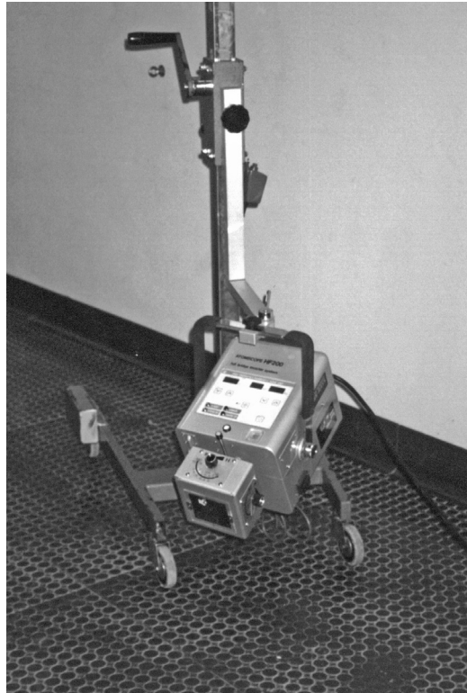
Figure 5.5 Typical design of a digital mobile X-ray unit.
